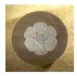
Material of the conductor: E-AlMgSi, crossection 95 mm², compacted thickness of the sheath (XLPE) 2,3mm
